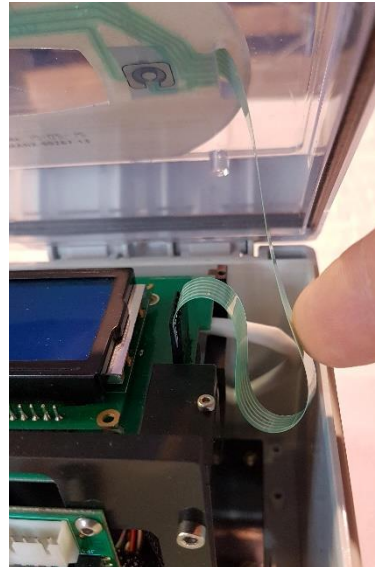
Figure 34 - Guide Ribbon Cable into the Enclosure
